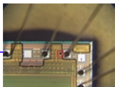
IC/wafer inspection at 200x
