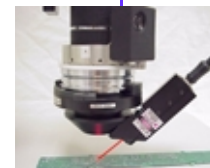
AD-5030SL 50x-300x with Laser Slit Light, Snap-On design For Solder Paste Height and Volume Measurement Precision +/- 12 micron at 50x to +/- 2 micron at 300x
