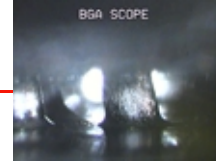
Deformed BGA ball & quick inspection for bridging
